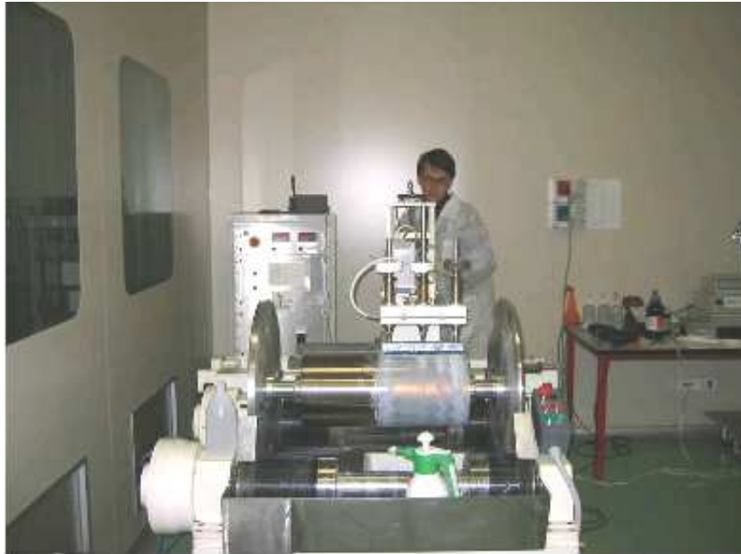
Figure 6.1: A Zeiss superpolishing machine at work on a Ni-coated mandrel.
