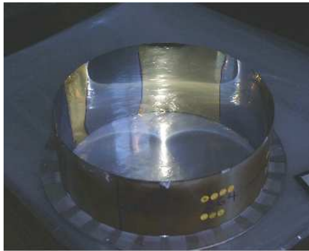
Figure 8.6: The mirror shell produced at the CfA and tested at the PANTER facility. The shell is a single cone with 280 mm maximum diameter, 20 m focal length, 125 mm height. The on-axis incidence angle is 0.21 \text{ deg} . The coated sectors on the Au background are clearly seen.
