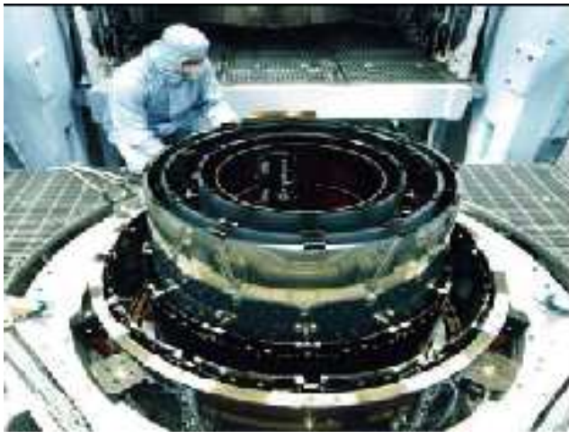
Figure 2.11: (left) The Chandra monolithic mirrors of the Chandra satellite during the assembly (credits: NASA). (right) The overall scheme of the Chandra telescope: the optics are visible in the front of the satellite (credits: NASA).
