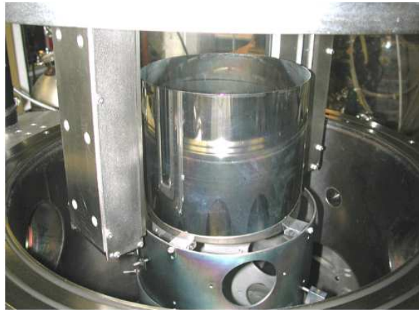
Figure 8.5: Inside the CfA DC magnetron coating facility. The facility is a cylinder 112 cm high, and 56 cm diameter, cryopumped down to 10^{-7} torr. Two linear cathodes (66 cm) are mounted in the center of the chamber: the optic is mounted around the cathodes. During the sputtering, the cathodes rotate to coat the inner side of the shell. A system of shutters allows the deposition of an element per time (credits: bibl. [89]).
