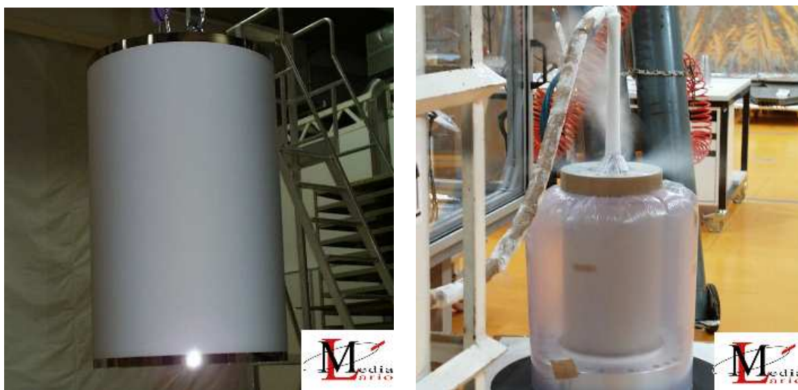
Figure 7.21: (left) The coated mandrel as in figure 7.20, after the Nickel electroforming. The Ni mirror wall was been grown on all the mandrel surface, except on the two terminal strips that were covered by the peelable paint (credits: Media-Lario s.r.l., cited with permission).
