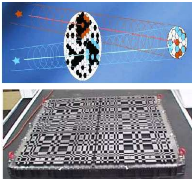
Figure 2.17: (top) Working principle for coded masks for hard X- and \gamma -rays. (bottom) An image of a real coded mask: the IBIS mask on-board INTEGRAL. (credits:ESA)
