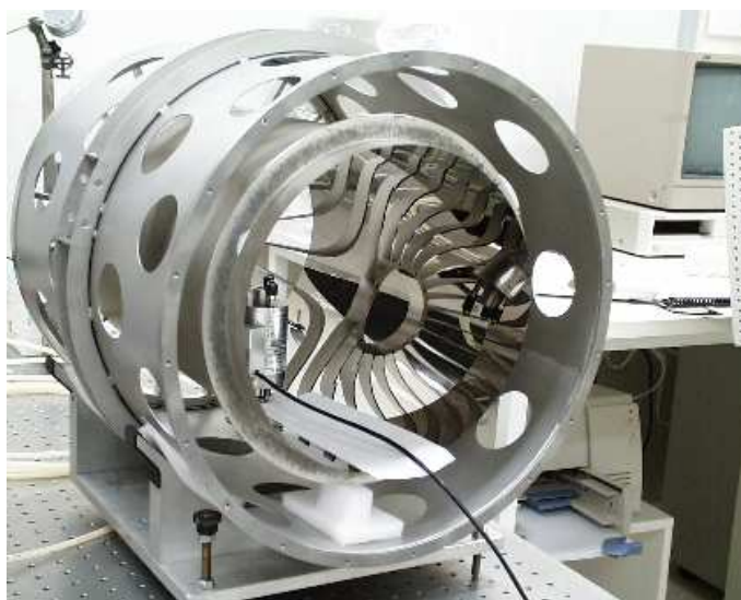
Figure 7.22: The integrated mirror shell in the case: the rear spider structure is visible, reflected on the mirror shell. The AFM has been installed on the inner shell surface in order to measure the surface microroughness.
