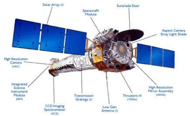
Figure 2.11: (left) The Chandra monolithic mirrors of the Chandra satellite during the assembly (credits: NASA). (right) The overall scheme of the Chandra telescope: the optics are visible in the front of the satellite (credits: NASA).
