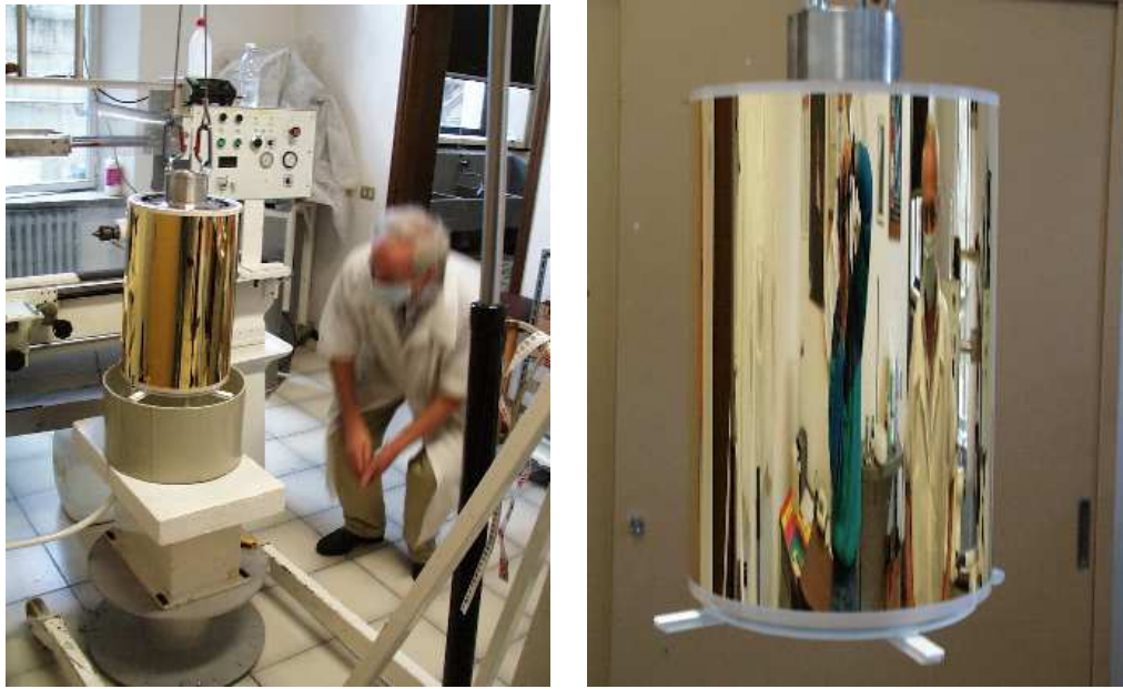
Figure 7.20: (left) Peelable paint application to the mandrel after Au + Pt/C multilayer + Cr + Au coating. Some centimeters of mandrel length are covered with a paint that isolates the coating from the electroless Nickel, making easier the release process. (right) The mandrel after the paint application. The visible coating is a 100 nm thick Au layer.
