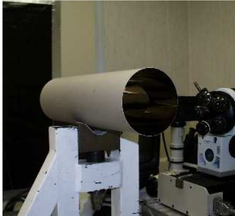
Figure 7.19: A Wolter I, Ni electroformed replicated mirror shell with 70 cm length and 12 cm diameter. The mirror shell has an inner coating of a Pt/C multilayer with 7 nm of capping Au.
