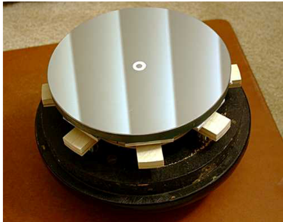
Figure 2. Mike Connelley's manually adjusted active primary mirror. Note the 8 wooden flex fingers.
