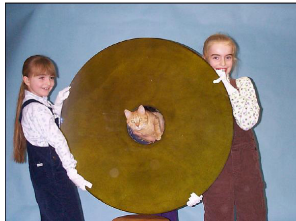
Figure 6. Carbon fiber composite mirror. The cat weighs more than the mirror. New mirror materials now allow much larger temperature changes.
