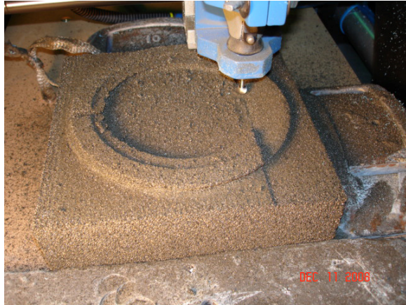
Figure 5. Foamglas puck being machined by Andrew Arigema. Plate glass can be fused or cemented to the finished pucks. Still highly experimental.
