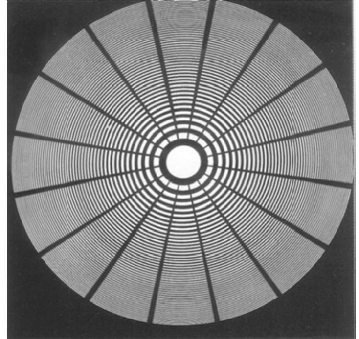
Radius  $n^{\text{th}}$  zone:  $r_n \simeq \sqrt{n f \lambda}$ , with  $N = n_{\text{max}} = \text{large} \rightarrow$
