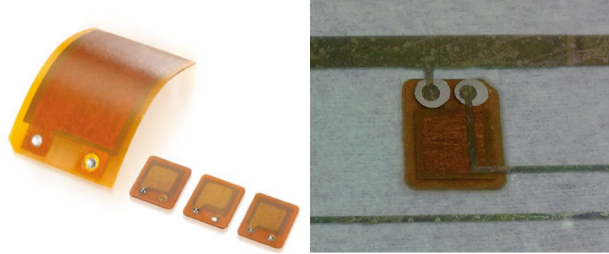
Figure 9.2: : Left: two models of the selected piezoceramic transducers. Right: a detail of the glued piezoelectric patch seen through an uncoated glass foil. The electrical contacts are ensured via two droplets of conductive epoxy.
