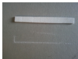
Figure 7.18: : Residuals left on cardboard when cutting a strip of Zirconia ZYF/100.
