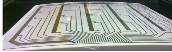
Figure 9.1: : The glass foil laying on the cylindrical slumping mould in K20, just after the slumping process. In this case the electrodes have been deposited on the flat glass, prior the slumping.
