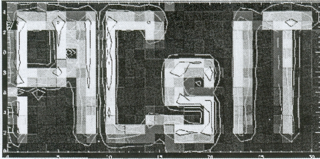
Figure 1: PICsIT QM response to ^{203}\text{Hg} photons (279 keV) obtained with a Pb mask in the shape of the word "PICsIT" placed between source and detector.
