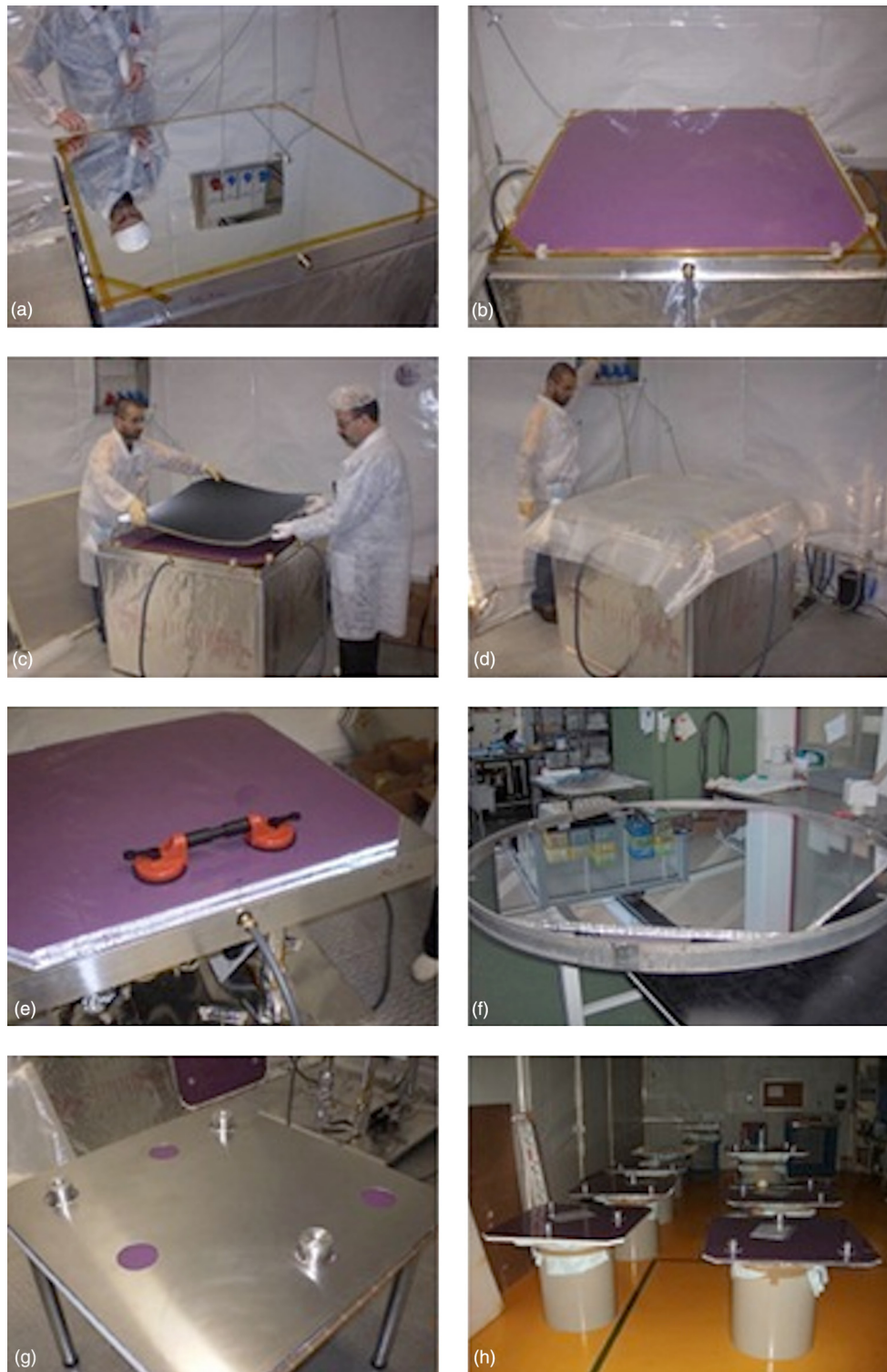
Fig. 8 Main steps of the manufacturing: (a)–(c) sandwich preparation; (d) polymerization of the glue; (e) sandwich release; (f) coating; (g) and (h) mirror's interfaces fixation and edge finishing.
