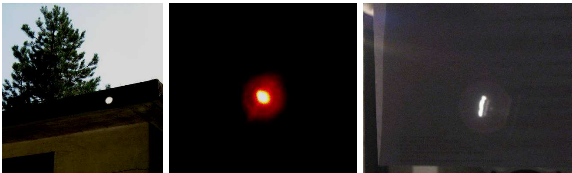
Fig. 4. Images generated by the prototype mirror panel realized: (left) an image of the Sun disk, (center) the focal spot on the radius of curvature and (right) a filament lamp.
