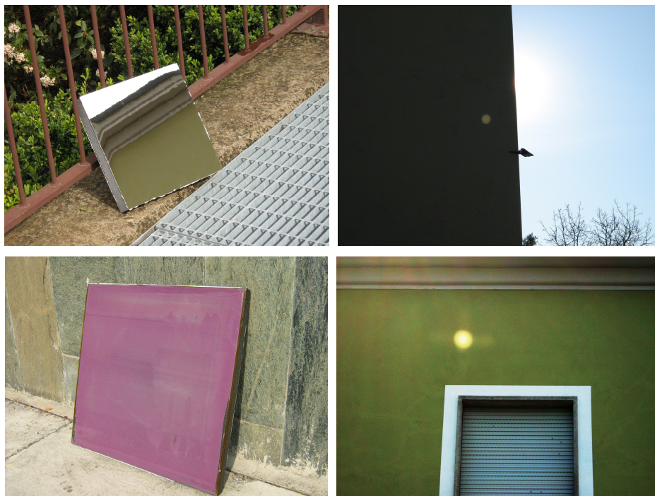
Fig. 9: Prototypes made with F-type Foamglas® core. (top-left) 300x300 mm 2 prototype, the surface is aluminized. (top-right) Image of the Sun generated by the small prototype. (bottom-left) 600x600 mm 2 prototype, the surface is not aluminized. (bottom-right) Image of the Sun generated by the larger prototype.
