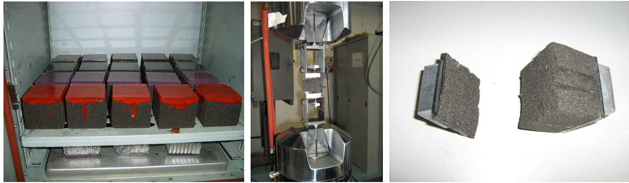
Fig. 6: (left) specimens during the curing of the glues (center) specimen mounted on the traction machine (right) specimen after the test.
