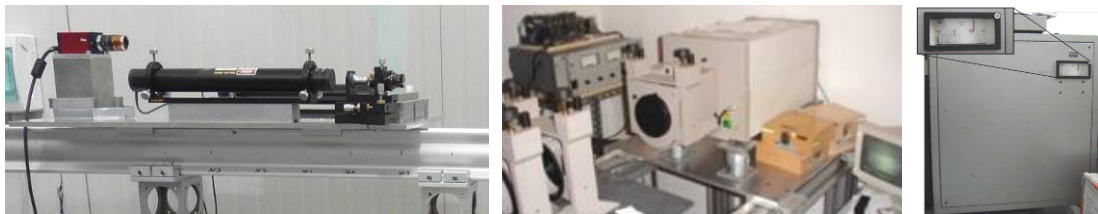
Fig. 5. Instrumentations used for the measurements of the mirror panel prototypes. From left to right: horizontal optical bench for focal spot measurement (laser source, lens and pinhole for spherical wavefront generation, CCD camera for image acquisition), 100 mm ZYGO GPI-XP interferometer and chamber for thermal cycling.
