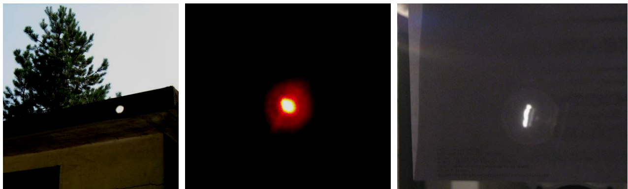
Fig. 12. Images generated by the prototype mirror panel realized: (left) an image of the Sun disk, (center) the focal spot on the radius of curvature and (right) a filament lamp.
