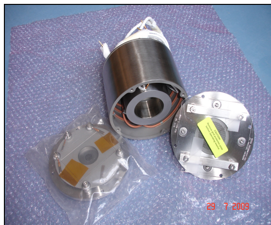
Fig. 7 Grids of the Ion Source: 50 (right) and 15 mm (left) diameter
