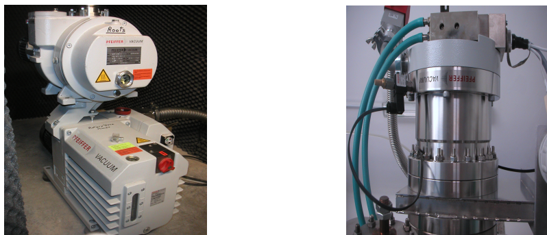
Fig. 3. Rotary and Roots pumps on the left side and one of the two turbo-molecular pumps for high vacuum on the right one
