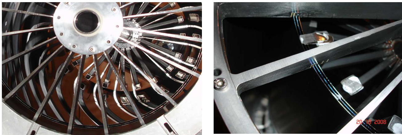
Fig. 1:(left) a view of the EM3 during the integration. Notice the mutual closeness of the 3 mirror shells. (right) the final stage of the integration of the mirror shells. The temporary clamps, utilized to endow the shells with the necessary stiffness while handled, are being removed.
