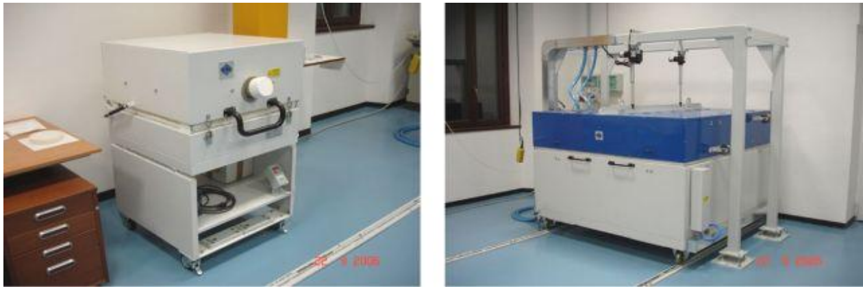
Fig. 4: Hot slumping facility available at INAF-OAB. The facility is composed by two ovens, a small one (left) and a big one (right) able to host moulds up to 1.1 m in diameter, a clean room environment for the preparation of the samples and a crane for the handling of weights up to 500 kg.
