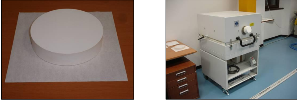
Fig. 2: (left) ZERODUR K20 mould used for tests. (right) Small oven for tests.
