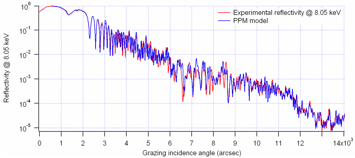
Fig. 11: reflectance plot at 8.05 keV of multilayer witness mirror. Logarithmic plot. The agreement of data (red line) with model (blue line) is satisfactory.
