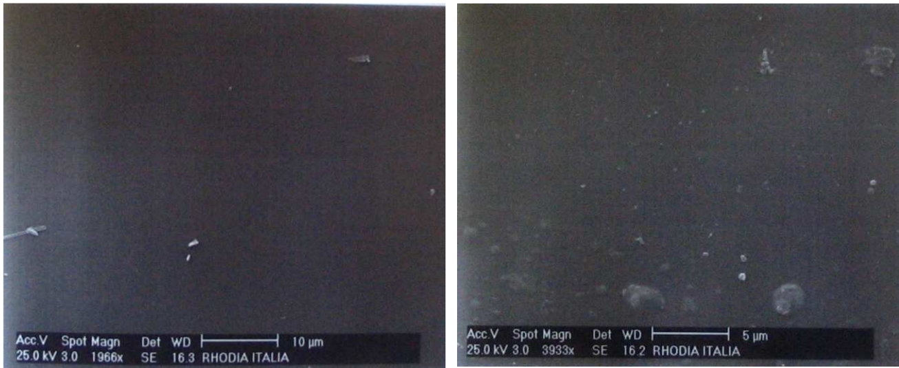
Fig. 13: SEM images of the surface of a PECVD SiC chip. (left) a major surface extent does not exhibit apparent surface features on 10 \mu\text{m} scales. (right) a minor surface extent is covered by small defects in ejection (courtesy by Rhodia Italia, Ceriano Laghetto, Italy).
