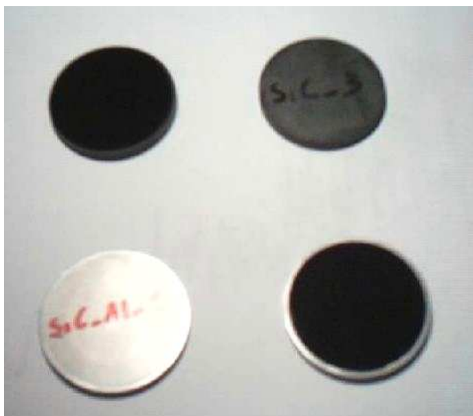
Fig.1: The samples being characterized in the present document. (top) two samples with Silicon Carbide substrates, (bottom) two samples with substrates in Aluminum. The SiC claddings have been deposited with the PECVD technique.
