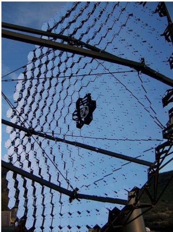
A VERITAS telescope (here: T4) showing the facet structure of the reflector.
