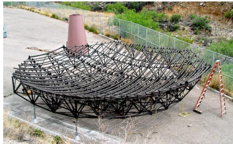
A VERITAS telescope (here: T4) showing the facet structure of the reflector.
