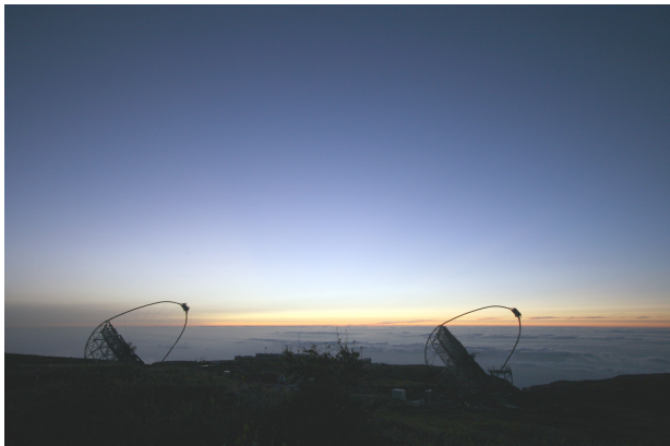
Stereo system at Canary Islands, \sim 80 m separation, camera \sim 1000 pixels (upgrading M-I)
