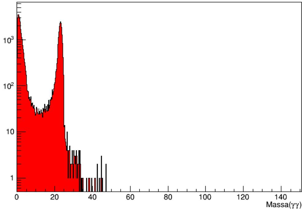
MC invariant mass for  $\gamma\gamma$  in time in the PADME Ecal ( $\sim 1e10 e^+$ ).
