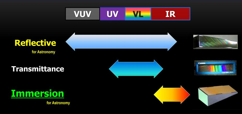
An Immersed grating is the absolute and simple solution of the downsizing concept in the high-precision infrared Spectroscopy.
