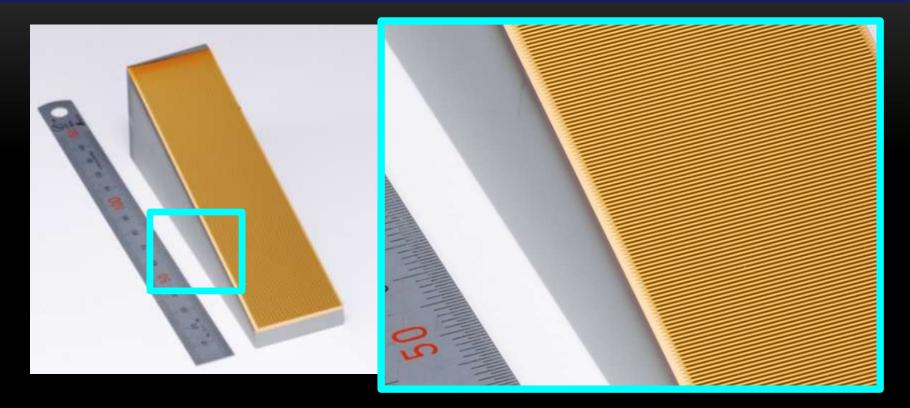
Grooved pitch: 476um for 3-5um Blaze angle: 75 degrees Maximum Absolute Diffraction Efficiency: 78%@ 4um
