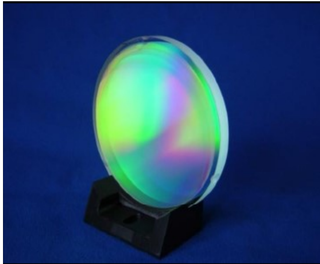
800gr/mm, D135mm transmission NIR grating (EMIR)
