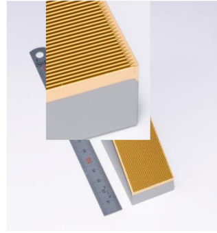
Fig.3 The picture of Germanium grism by machining with 2.2 \mu m pitch.
